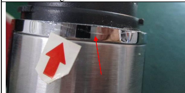
66. Defect: Scratched on decorative ring
