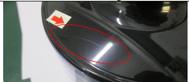
69. Defect: Scratched on lid
