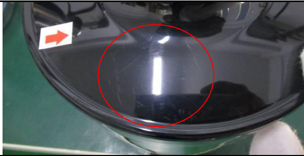
72. Defect: Scratched on lid
