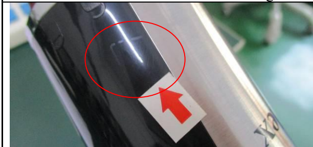
68. Defect: Scratched on unit
