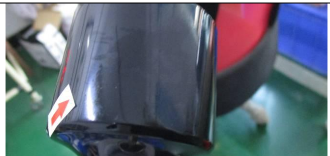
71. Defect: Oil on whisk holder
