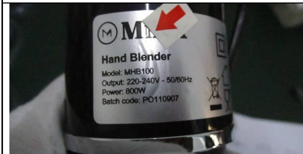
70. Air bubble on rating label
