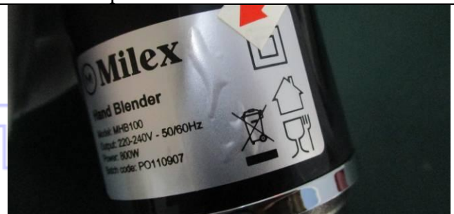
67. Defect: Air bubble on rating label
