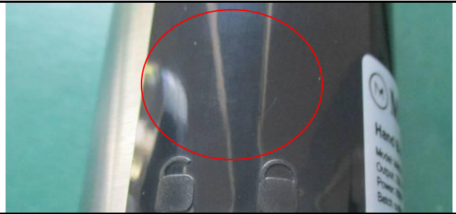
73. Defect: Scratched on unit
