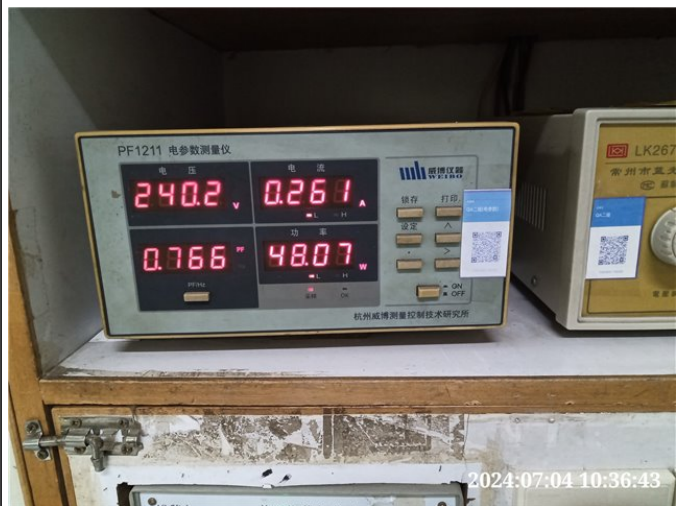
Photo# 98 Power consumption test(motor appliance)
