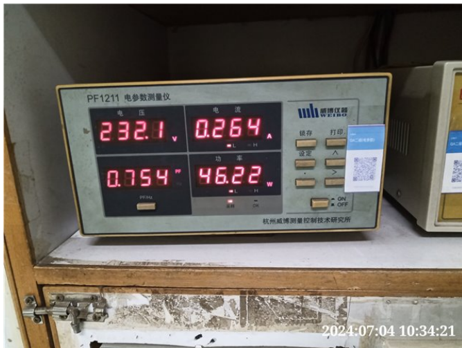
Photo# 91 Power consumption test(motor appliance)
