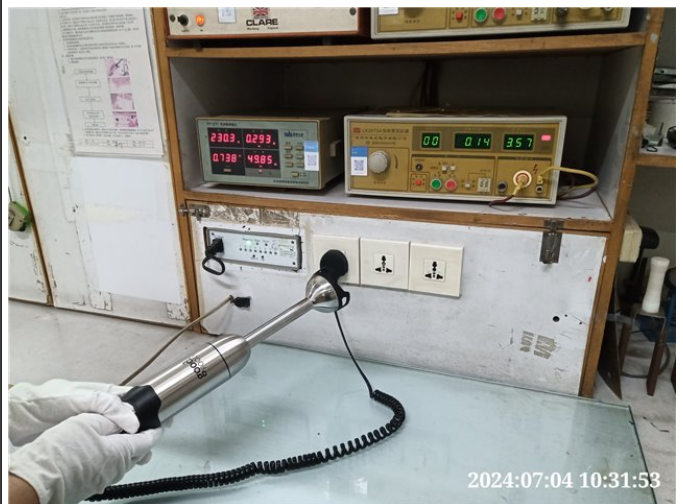
Photo# 86 Power consumption test(motor appliance)
