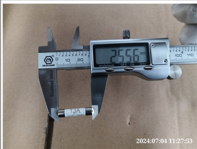
Photo# 211 Fuse check
