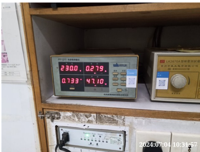
Photo# 87 Power consumption test(motor appliance)
