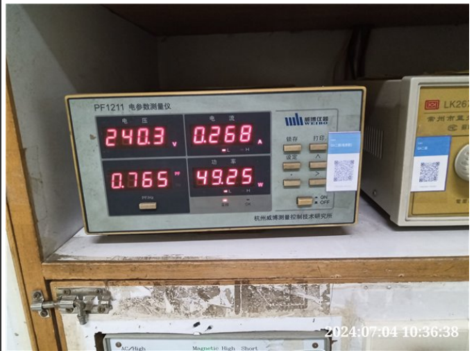
Photo# 96 Power consumption test(motor appliance)
