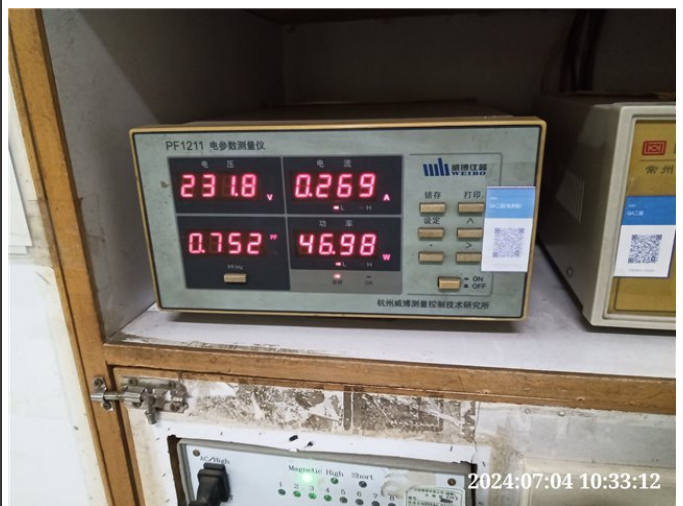
Photo# 88 Power consumption test(motor appliance)
