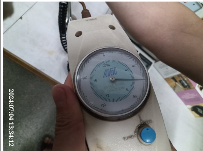
Photo# 29 Power cord strain relief test
