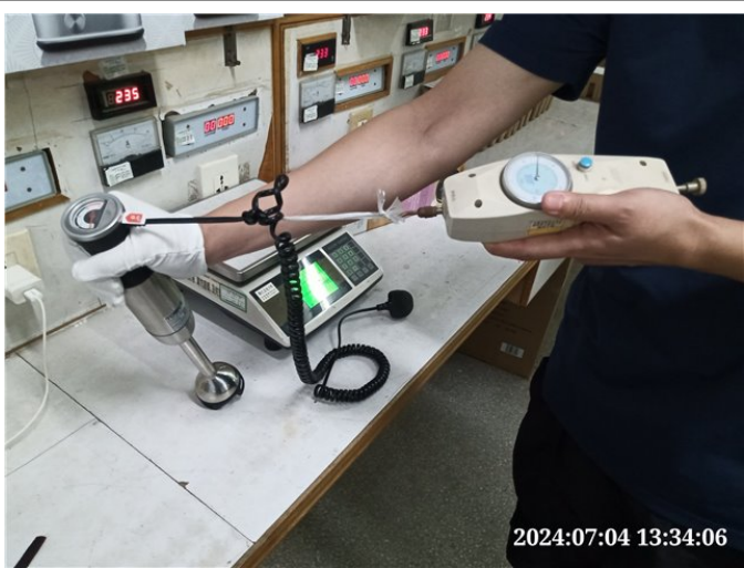
Photo# 28 Power cord strain relief test
