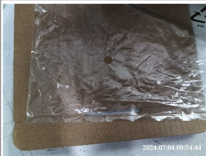
Photo# 171 Air hole
