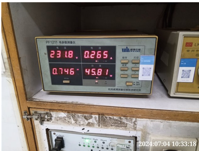
Photo# 89 Power consumption test(motor appliance)
