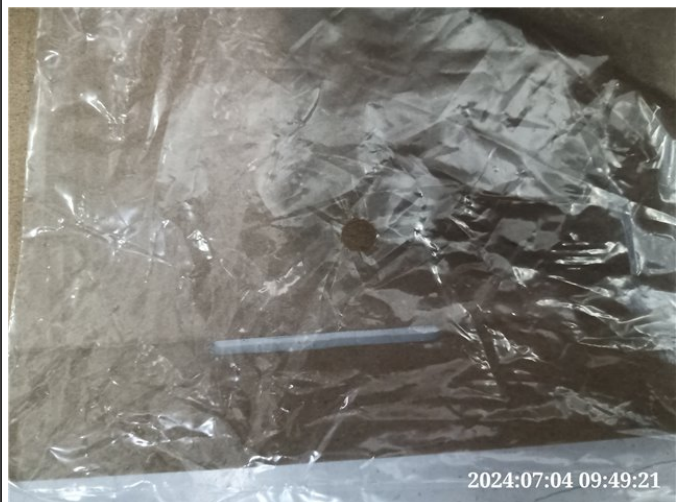
Photo# 150 Air hole
