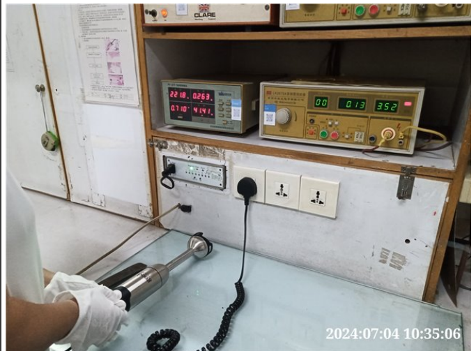
Photo# 92 Power consumption test(motor appliance)
