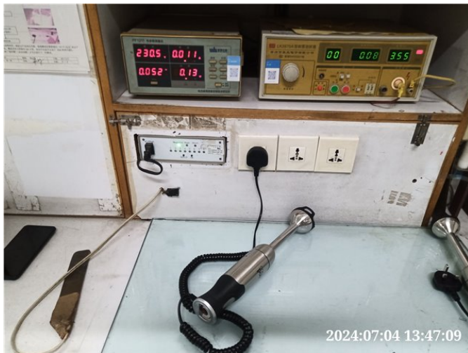
Photo# 83 Standby power/off power test
