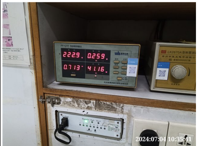
Photo# 94 Power consumption test(motor appliance)
