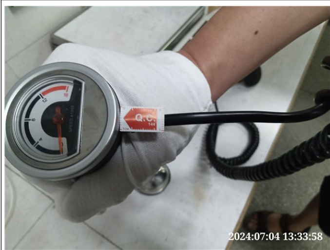
Photo# 27 Power cord strain relief test
